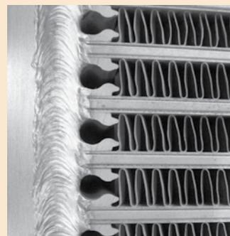
AKG-Line uses AKG hollow profiles to reduce local peak strains. This way the strength of heat exchangers is significantly increased and their service life time considerably prolonged.
