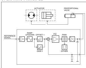
The EDM-M∗ card is a digital amplifier for open loop proportional valves control. It is designed for rail mounting type: DIN EN 50022.
