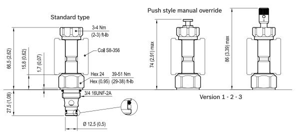
Version 2: Solenoid operated valve, poppet 2-way normally open Version 3: Solenoid operated valve, poppet 2-way double lock normally open
