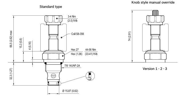
Version 2: Solenoid operated valve, poppet 2-way normally closed Version 3: Solenoid operated valve, poppet 2-way double lock normally closed
