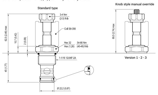
Version 2: Solenoid operated valve, poppet 2-way normally closed Version 3: Solenoid operated valve, poppet 2-way double lock normally closed
