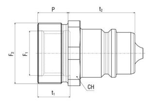
Male coupling - Internal/external thread panel mounting
