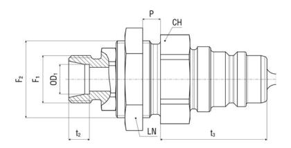
Male coupling - Metric 24° light/heavy series panel mounting
