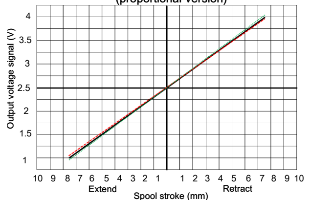
Output signal control characteristic (proportional version)
