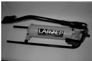
It has oil level, base structure of great stability, quick-connect male coupling and operating pedals de both for loading and unloading operations. (Free hands)
